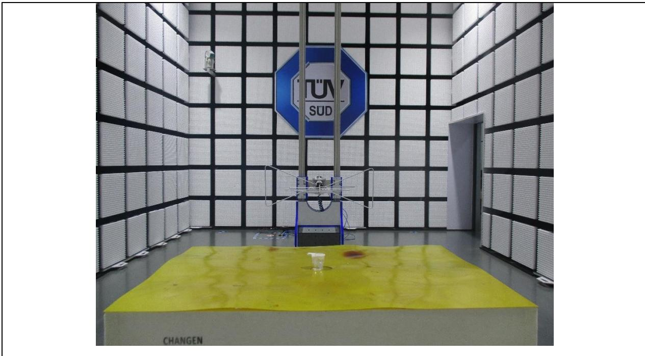
Details of: Radiated Emission test (1-18GHz)
