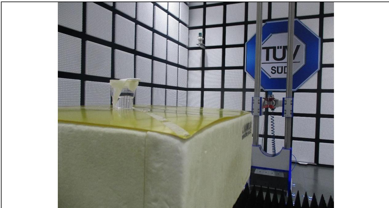
Details of: Radiated Emission test (18G-40Hz)
