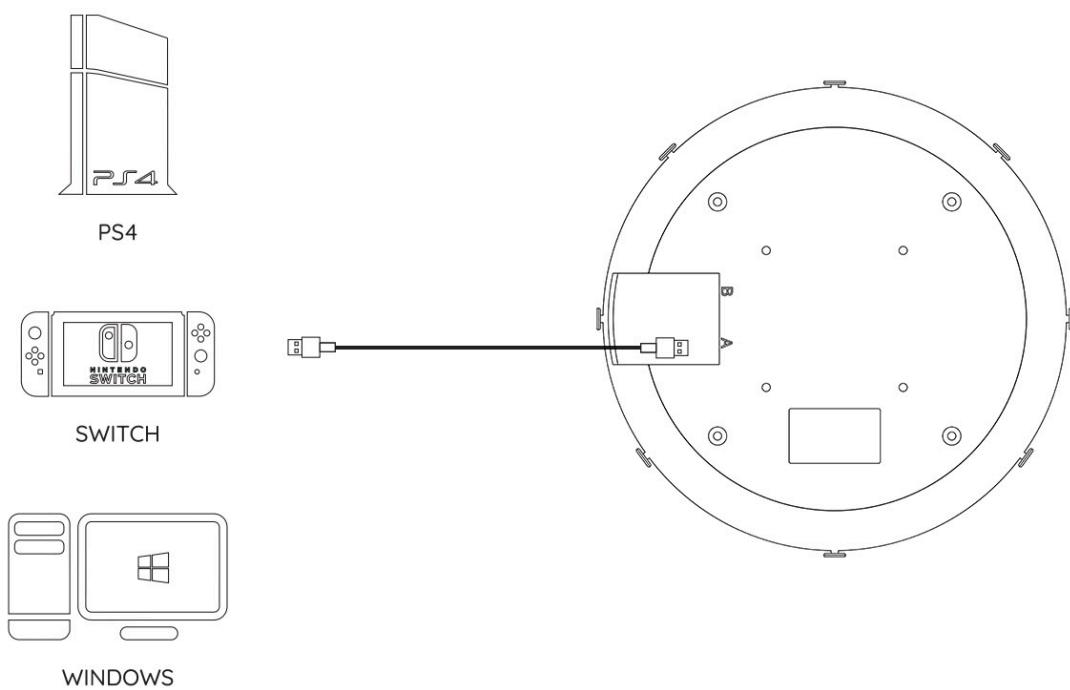
Use provided USB cable, connect port A on TDC-10 to USB port on game device, which usually used for connect standard game controller. TDC-10 is a kind of low energy device. In general, direct USB connection could get enough power for TDC-10 to run. For Switch and PS4, please make sure following corresponding tips below.
