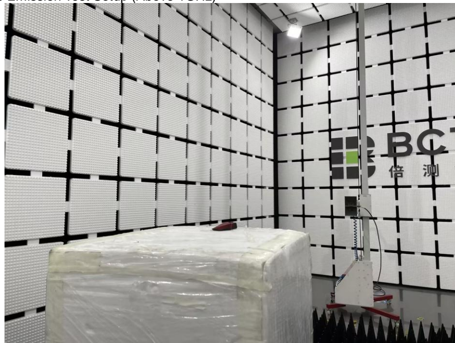
Spurious Emission Test Setup (Above 1GHz)
