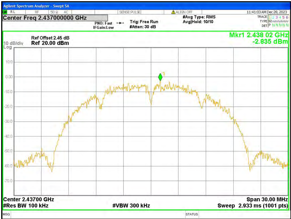
Tx. Spurious NVNT b 2437MHz Ant1 Ref
