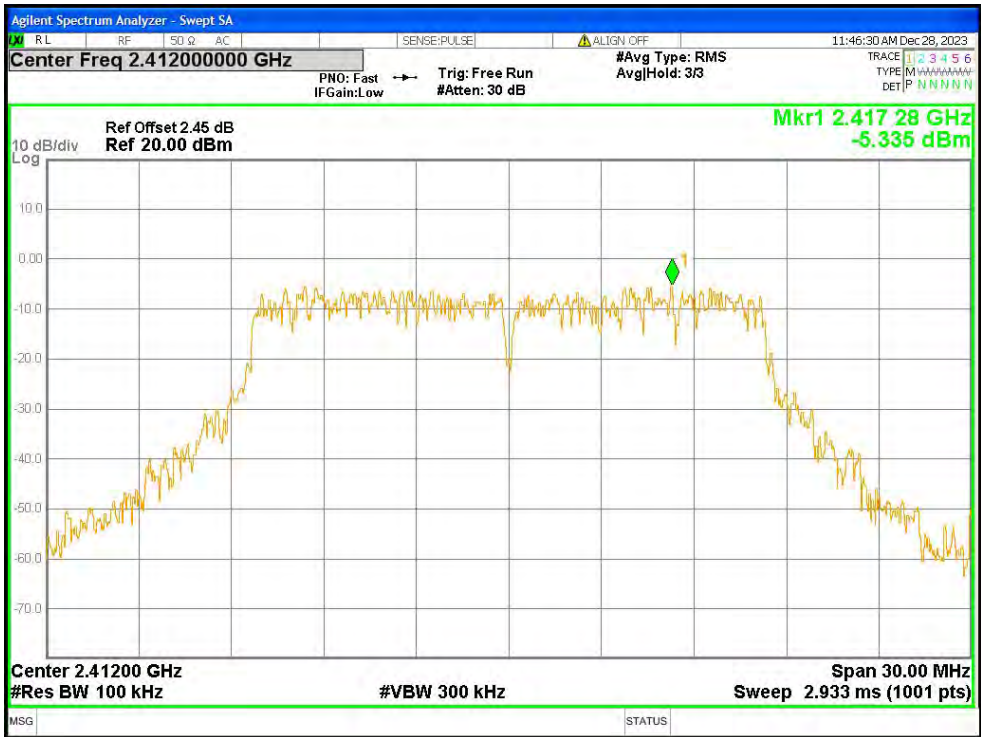
Tx. Spurious NVNT g 2412MHz Ant1 Ref
