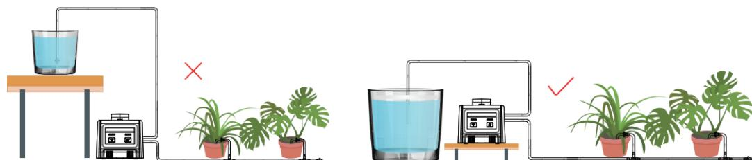
2.2 The lift length of the water pump: the vertical distance of 2-3m, because the water pipe can not be placed 100% straight, we recommend that the height between the plants and pump should not exceed 2.5m.
