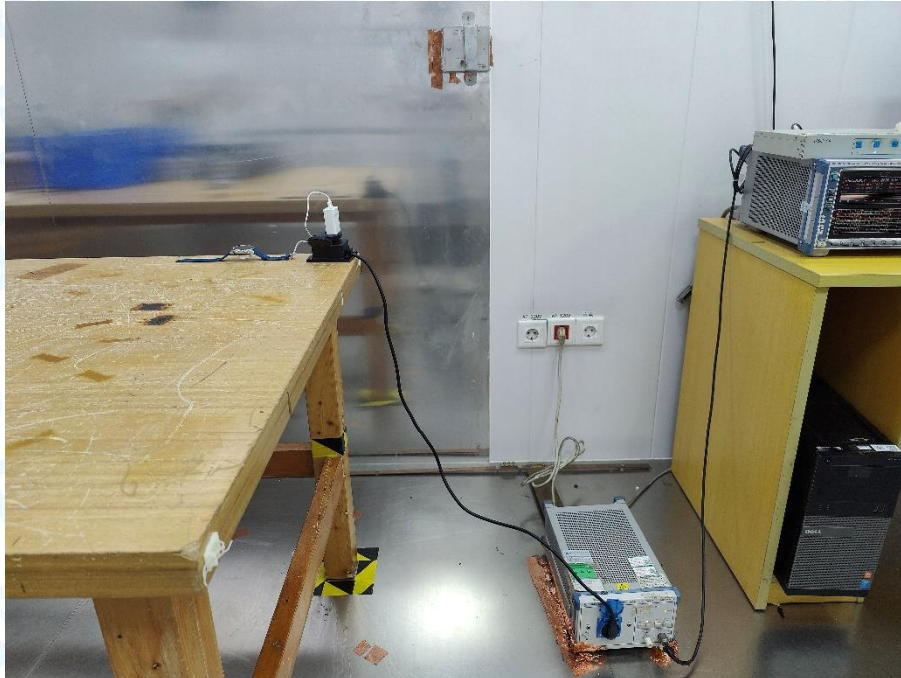
Photo of Setup for Radiated Emission (30MHz~1GHz)
