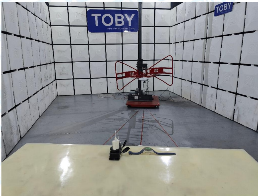
Photo of Setup for Radiated Emission (30MHz~1GHz)
