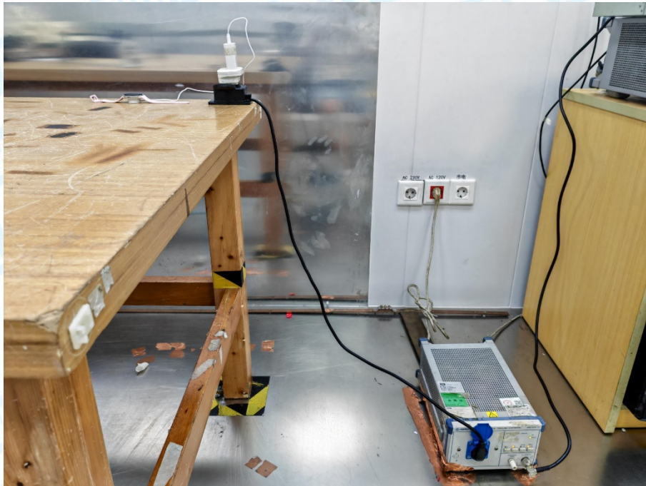
Photo of Setup for Conducted Measurement
