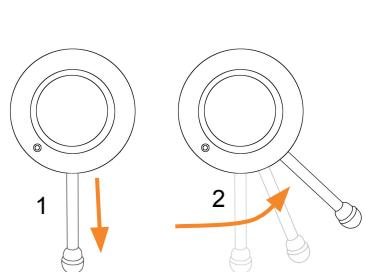
Pull out and push the tripod mount handle to the right to unlock the adapter.
