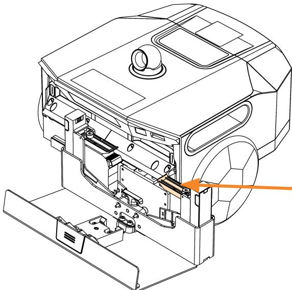
Once the print stall has been moved to one side, raise the cartridge latch to gain access to the ink.
