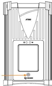
Power down the laser tracker by holding the power button for a few seconds. The screen will shut off indicating a power down.
