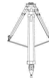
Remove the adapter from the tripod. **Lower the tripod legs**, detach the stabilizer, and fold the tripod back to its original position.
