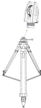
Carefully remove the head from the tripod. **Use both hands!**
