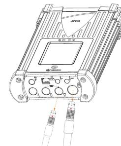
**Once the laser tracker is powered down, disconnect the cables and detach the controller and radio from the tripod.**
