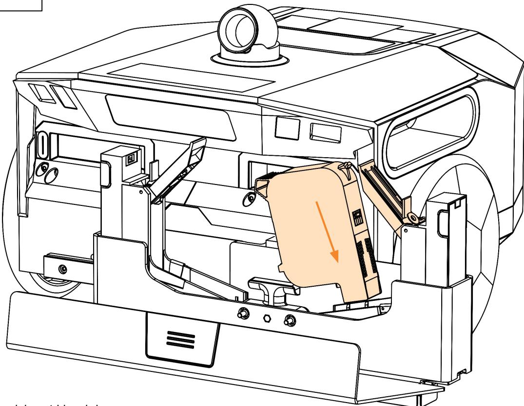
When placing the new ink cartridge, bring the cartridge in at a slightly diagonal angle like shown. **Try to ensure that the angle is as vertical as possible to prevent damage to the cartridge.** Hold the flap fully open while inserting the cartridge. Close the lever when the cartridge has been replaced.
