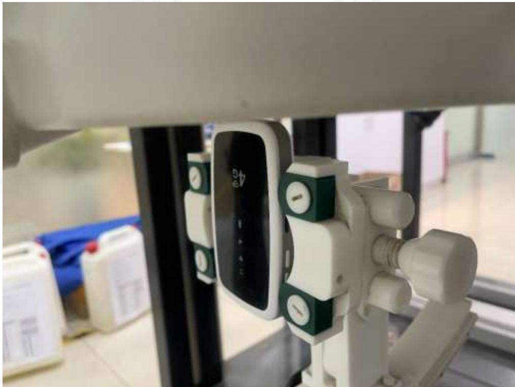
Limbs Bottom Side (separation distance is 0mm)
