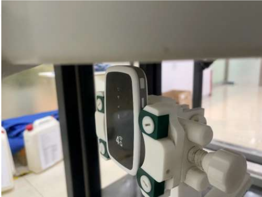
Body Top side(separation distance is 5mm)
