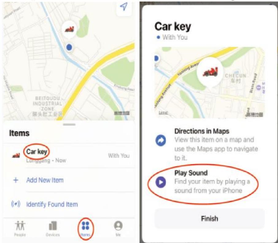
**Note:** When need to remove the device, please keep the device connecting with the Apple device, tap Play Sound can hear the slight noise of Di Di Di, then can make Remove.
