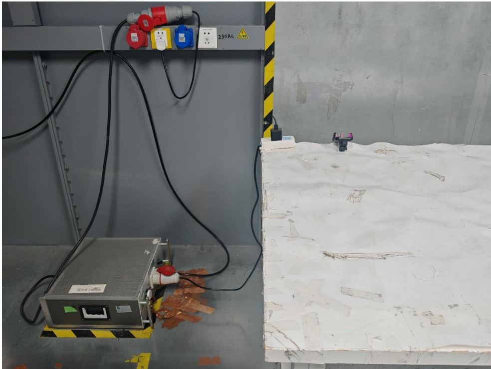
Photo of Conducted Emission test
