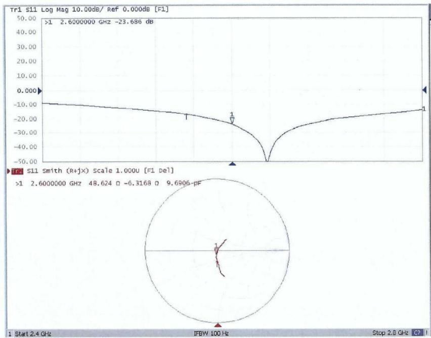
Referring to KDB 865664D01V01r03, if dipoles are verified in return loss (<-20dB, within 20% of prior calibration) and in impedance (within 5 ohm of prior calibration), the annual calibration is not necessary and the calibration interval can be extended.
