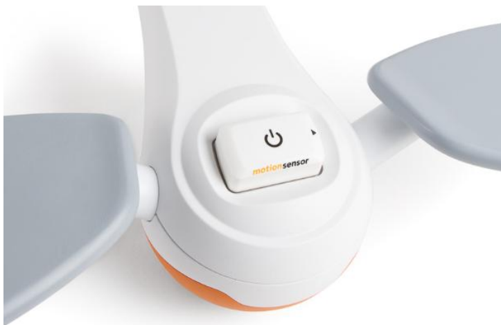
Figure 30: Correct alignment of the PABLO® Motionsensor on the PABLO® Multiboard
