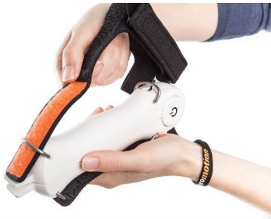
Figure 26: Fixation of the wrist strap - 1
