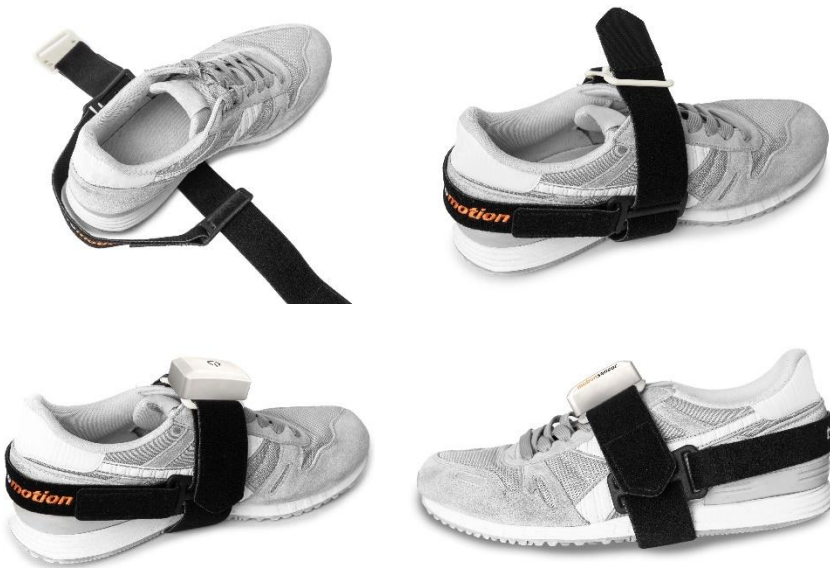
Figure 55: Fixation of the PABLO® Motionsensor on the foot with foot strap set
