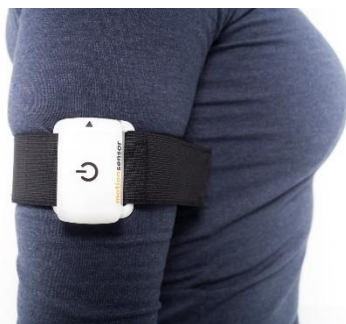
Figure 31: Correct alignment of the PABLO® Motionsensor in conjunction with straps
