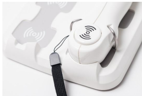
Figure 47: Wrong positioning of the sensors (NO charging!)
