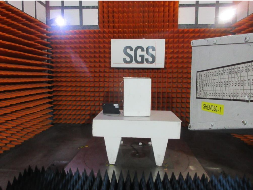
Radiated Spurious Emissions Above 1GHz
