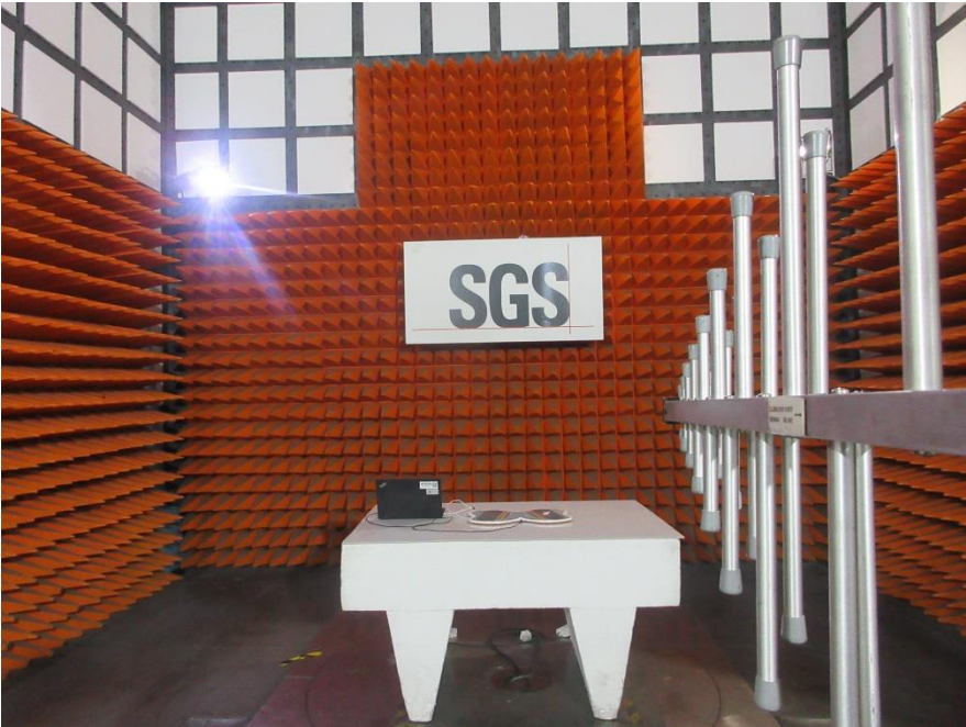
Radiated Spurious Emissions Below 1GHz
