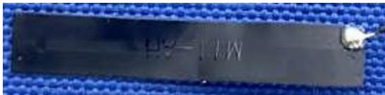
A photograph of a rectangular FPCB antenna. It is a dark grey or black rectangular component with a small white connector at one end. It is placed on a blue textured surface, likely a test fixture or a piece of cloth. |                   |
