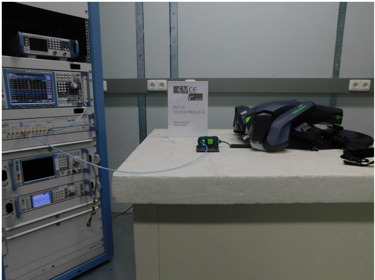
Conducted test setup - Regulatory Test System for Wireless Devices TS8997 / R&S
