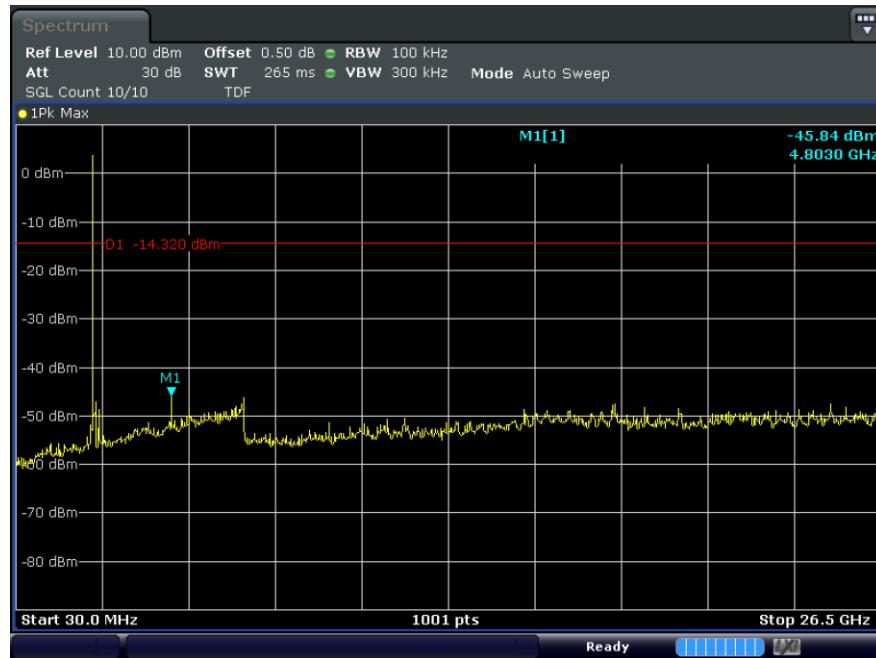
**B.1. Middle Ch. (2 440 MHz) Spurious emissions**
