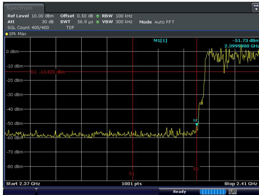
**A.3. Lowest Ch. (2 402 MHz)\_Spurious emissions**
