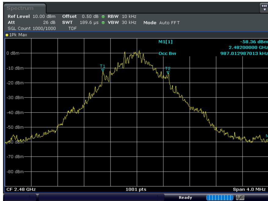
**Test mode : EDR****A.1. Lowest Ch. (2.402 MHz)\_20 dB Bandwidth**
