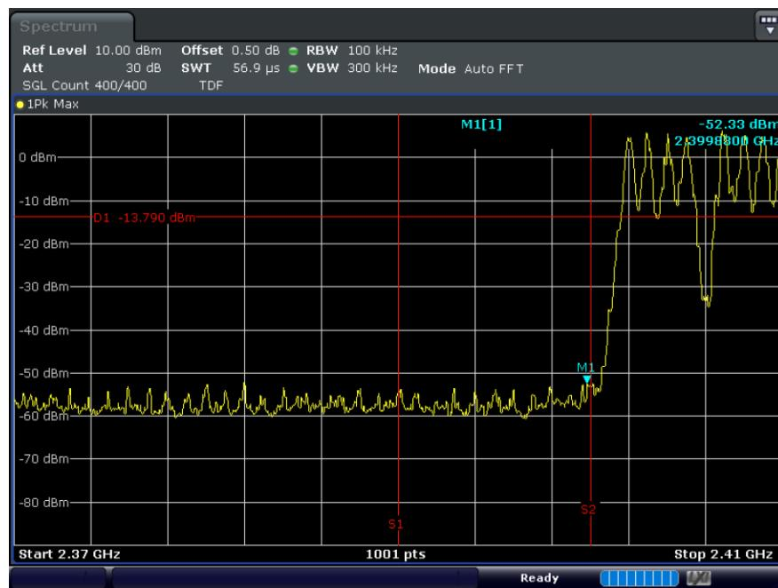
**A.3. Lowest Ch. (2 402 MHz)\_Spurious emissions**
