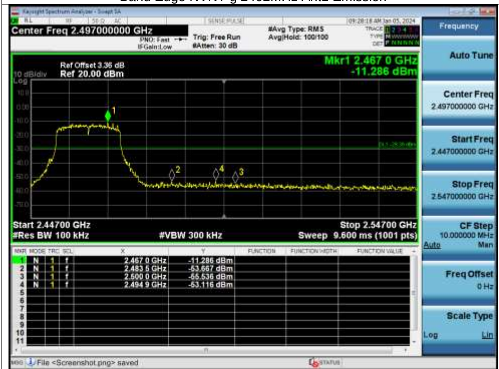
Band Edge NVNT g 2462MHz Ant1 Emission
