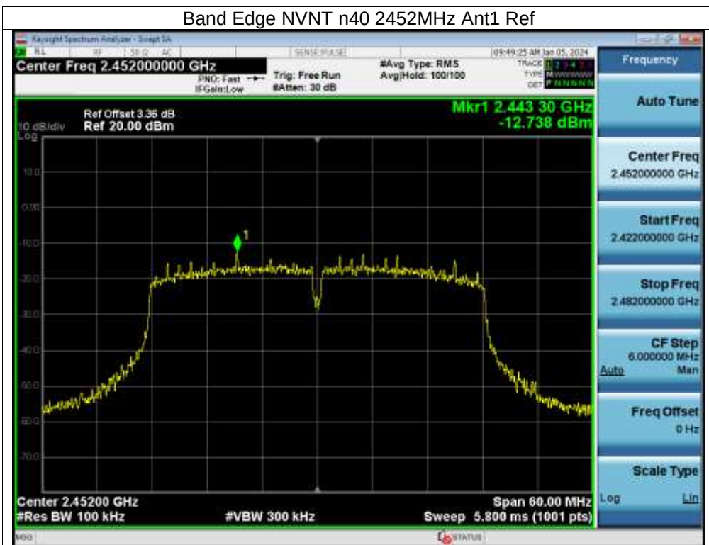
Band Edge NVNT n40 2452MHz Ant1 Emission
