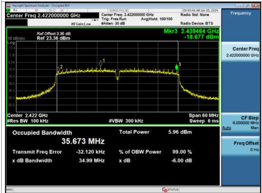
-6dB Bandwidth NVNT n40 2422MHz Ant1
