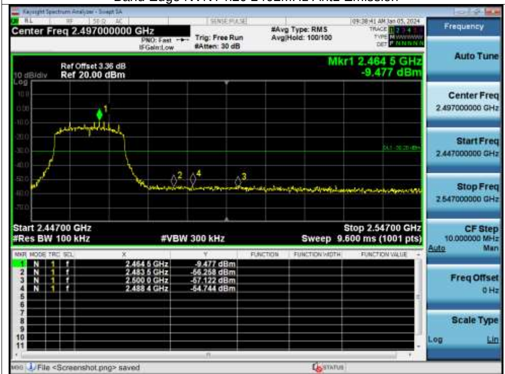
Band Edge NVNT n20 2462MHz Ant1 Emission
