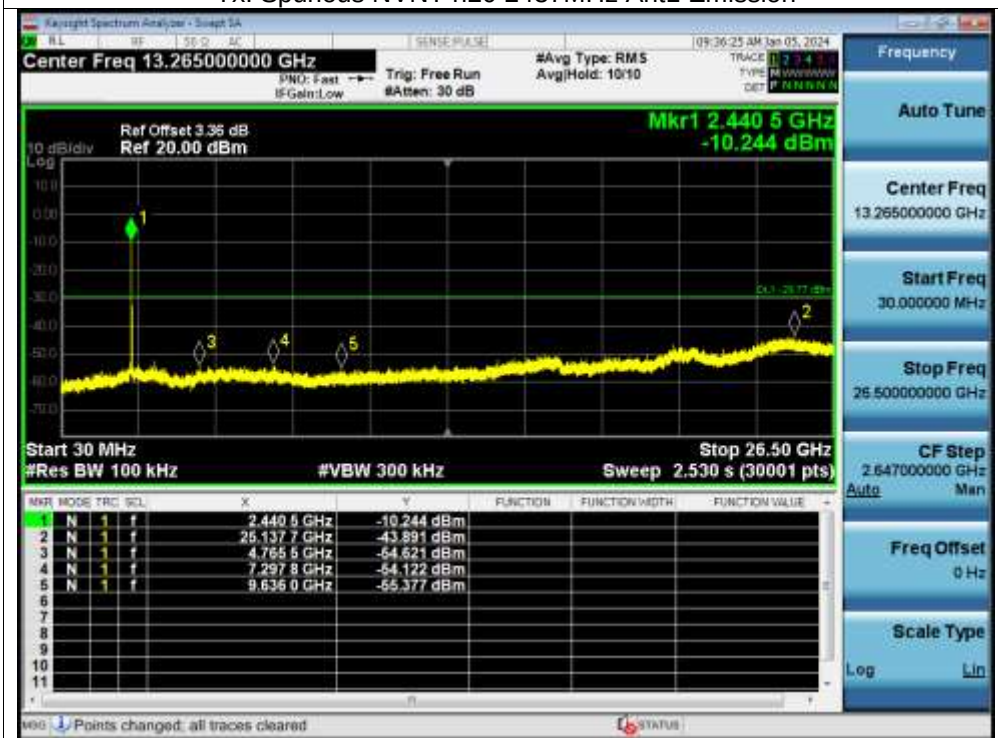
Tx. Spurious NVNT n20 2437MHz Ant1 Emission
