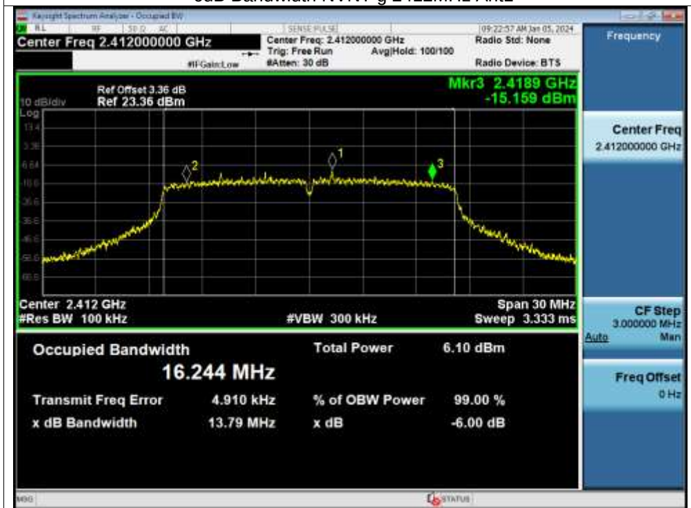
-6dB Bandwidth NVNT g 2412MHz Ant1
