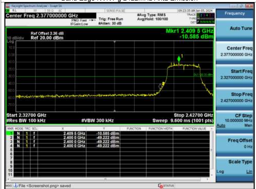
Band Edge NVNT g 2412MHz Ant1 Emission
