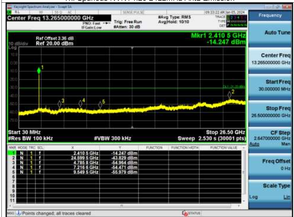
Tx. Spurious NVNT n20 2412MHz Ant1 Emission
