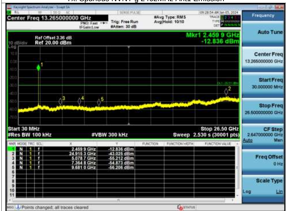
Tx. Spurious NVNT g 2462MHz Ant1 Emission
