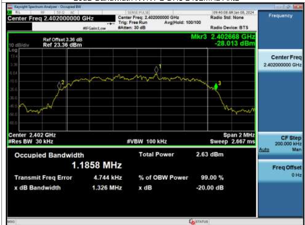
-20dB Bandwidth NVNT 2-DH5 2402MHz Ant1
