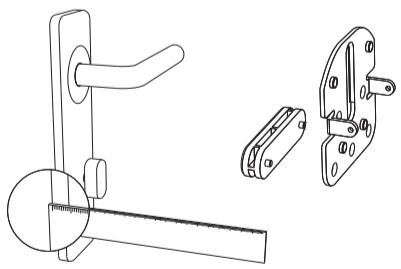
B3. Remove the screw 1 cm out from the door lock, aim the mounting plate into the card, align the center of the knob with the crossed red line, attach the mounting plate to the door, remove the card, and lock the screw back to its original positioning.
