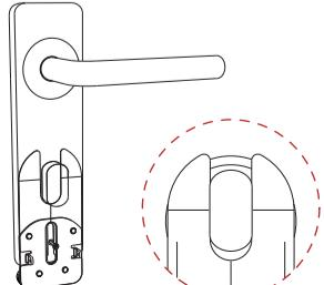
A3. Align the center of the knob with the crossed red line, attach the mounting plate to the door, and remove the card.
