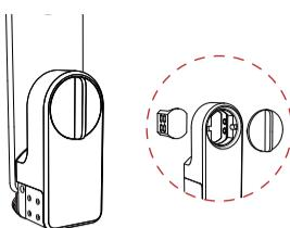
B9. Lock the screws on both sides.
