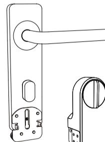
B7. Thin knob: Find the Clamp Gasket, fix it on the thin knob.
