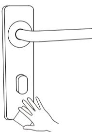
B2. Measure the thickness of the door lock, select the appropriate gasket and sticker, and attach it to the mounting plate.
