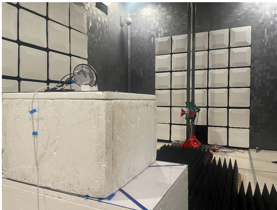
Figure 4 - Radiated emissions above 1 GHz (1 – 18 GHz), rear view.
