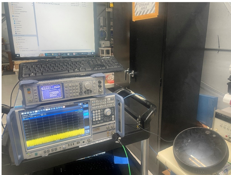
Figure 8 – Test setup (spectrum analyzer measurements)
