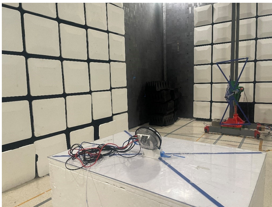
Figure 2 - Radiated emissions below 1 GHz (0.03 – 1 GHz), rear view.
