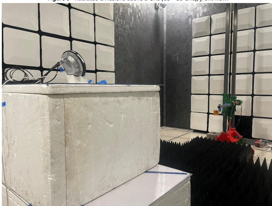
Figure 6 - Radiated emissions above 1 GHz (18 – 26 GHz), rear view.
