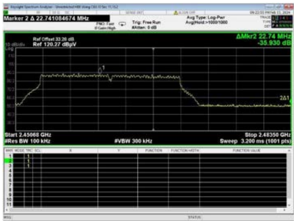
Figure 63 – Band-edge Measurement, WiFi G, High Data Rate, High Channel, Unrestricted Frequency
