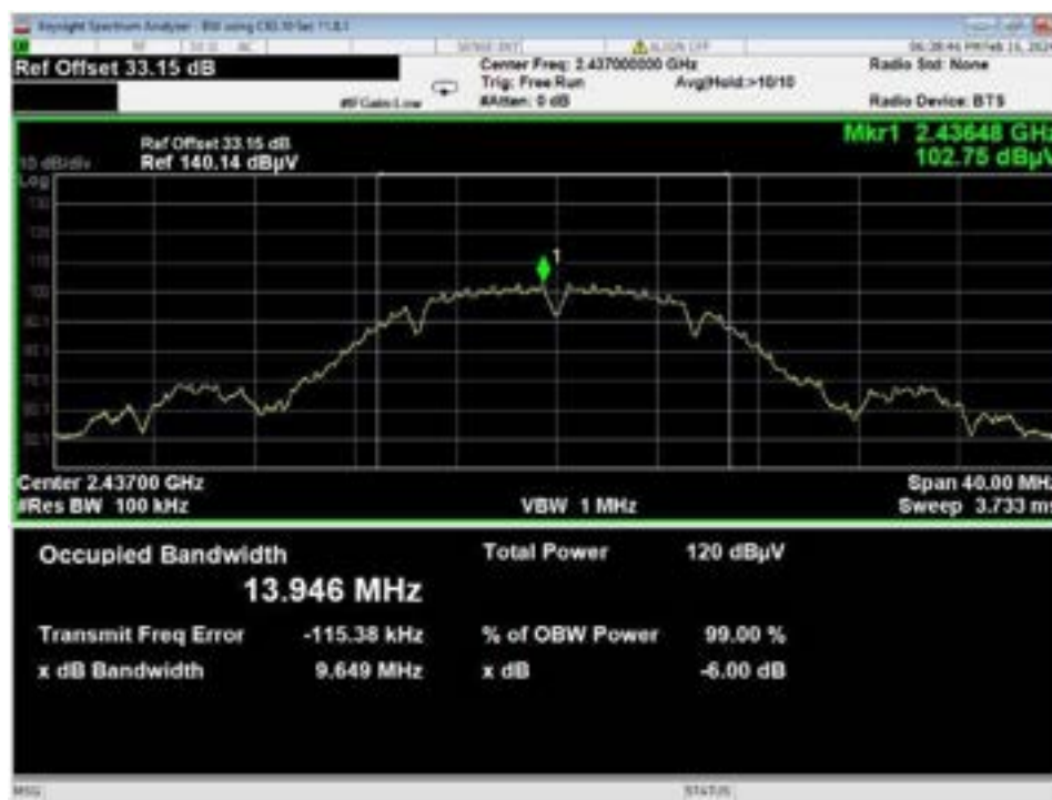
Figure 27 - Bandwidth, WiFi B, Low Data Rate, Mid Channel
