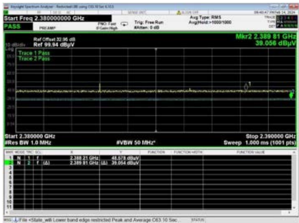
Figure 54 – Band-edge Measurement, WiFi N, High Data Rate, Low Channel, Restricted Frequency
