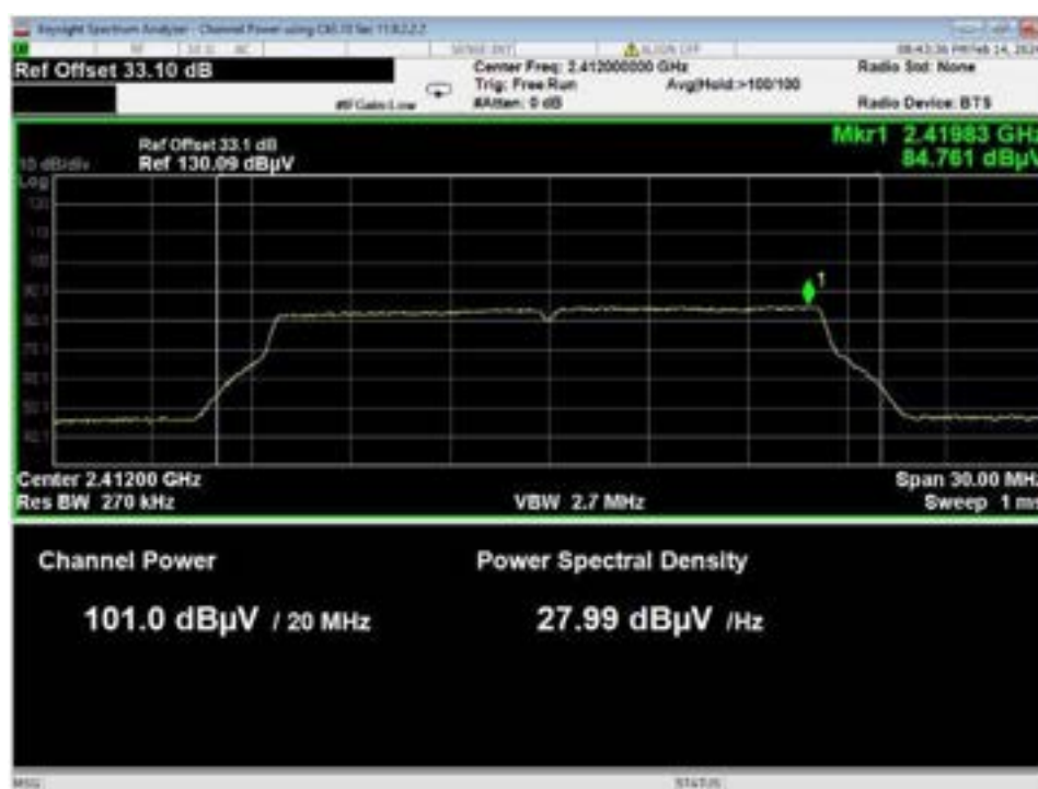
Figure 16 – Radiated Output Power Field Strength, WiFi G, High Data Rate, Low Channel.
