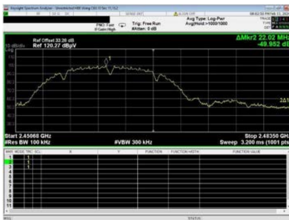
Figure 57 – Band-edge Measurement, WiFi B, Low Data Rate, High Channel, Unrestricted Frequency
