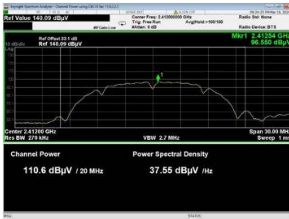
Figure 7 – Radiated Output Power Field Strength, WiFi B, Low Data Rate, Low Channel.
