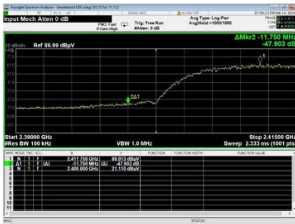
Figure 58 – Band-edge Measurement, WiFi B, High Data Rate, Low Channel, Unrestricted Frequency
