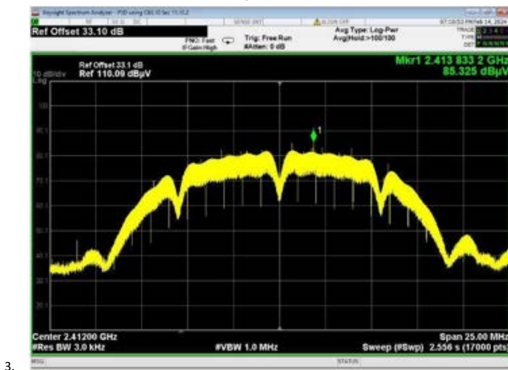
Figure 68 – Radiated EIRP Power Spectral Density, WiFi B, Low Data Rate, Low Channel
