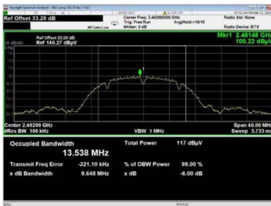
Figure 28 - Bandwidth, WiFi B, Low Data Rate, High Channel
