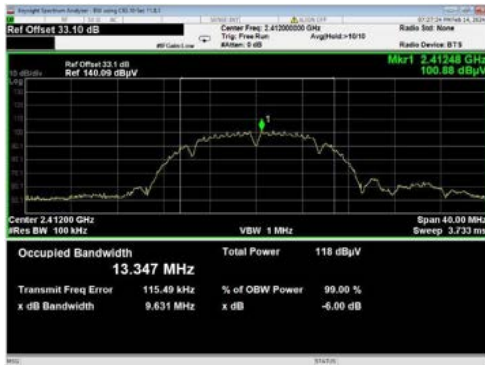
Figure 26 –Bandwidth, WiFi B, Low Data Rate, Low Channel
