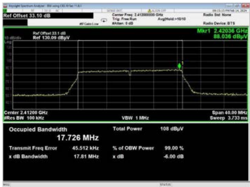
Figure 38 –Bandwidth, WiFi N, Low Data Rate, Low Channel
