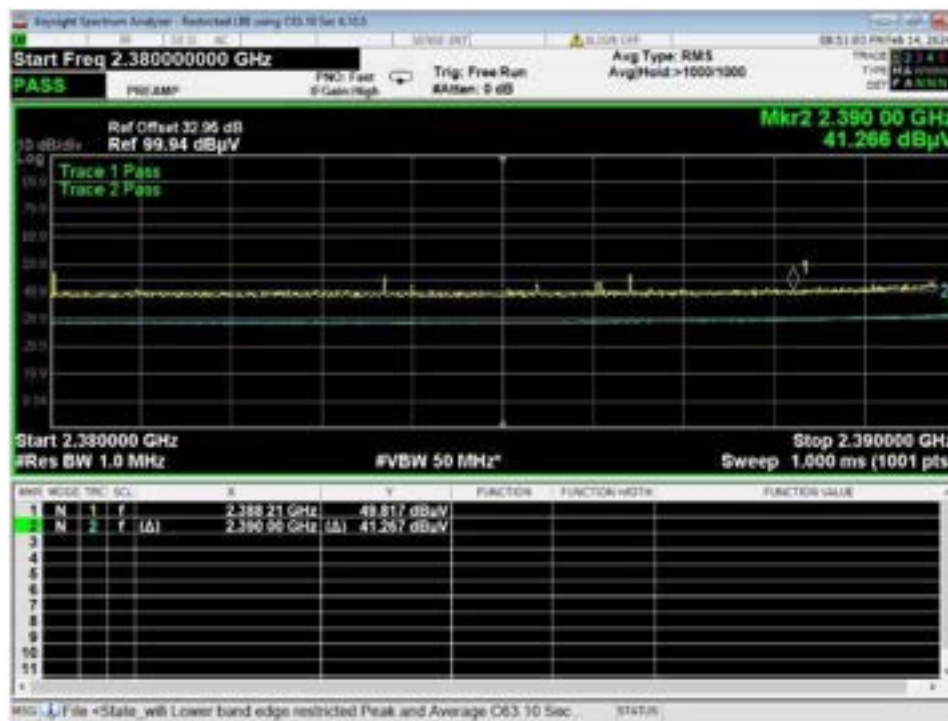
Figure 50 – Band-edge Measurement, WiFi G, High Data Rate, Low Channel, Restricted Frequency
