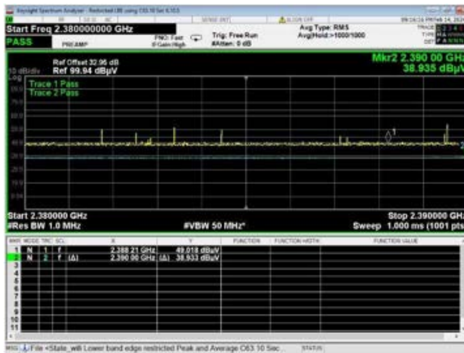
Figure 52 – Band-edge Measurement, WiFi N, Low Data Rate, Low Channel, Restricted Frequency
