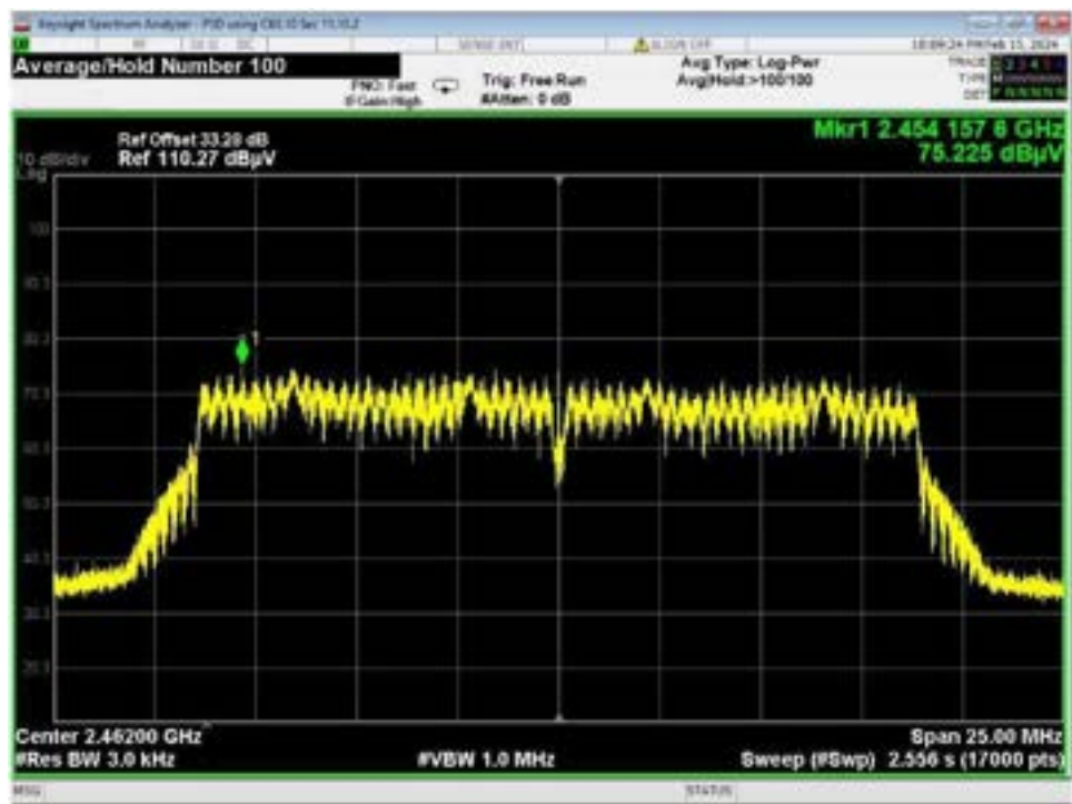
Figure 85 – Radiated EIRP Power Spectral Density, WiFi N, High Data Rate, High Channel
