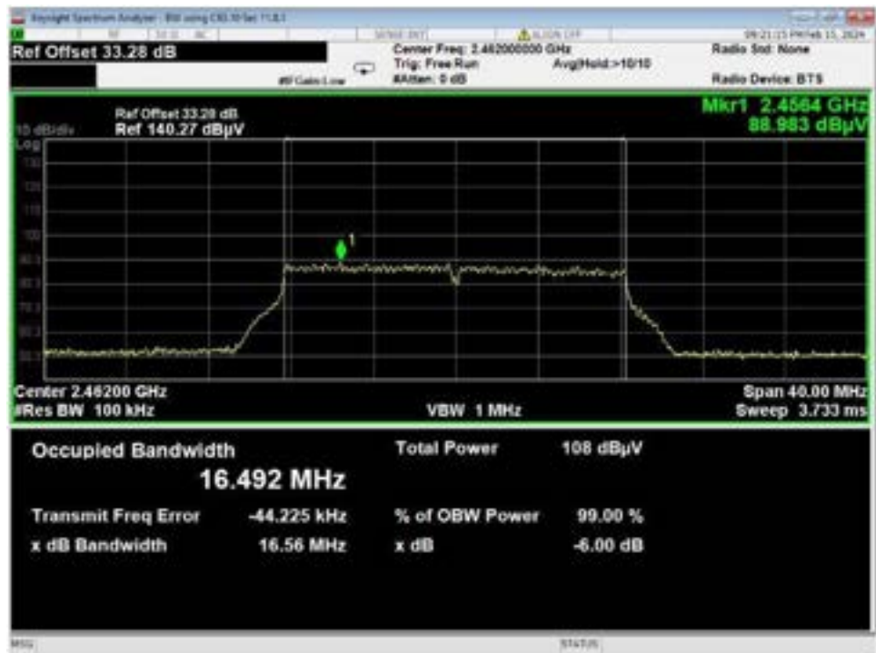
Figure 37 - Bandwidth, WiFi G, High Data Rate, High Channel
