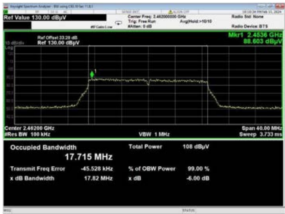
Figure 43 - Bandwidth, WiFi N, High Data Rate, High Channel
