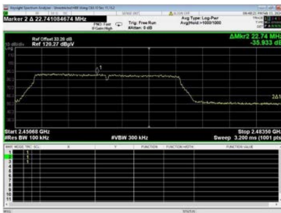
Figure 65 – Band-edge Measurement, WiFi N, Low Data Rate, High Channel, Unrestricted Frequency
