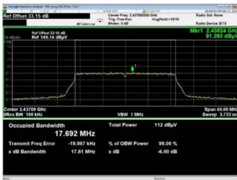
Figure 42 - Bandwidth, WiFi N, High Data Rate, Mid Channel
