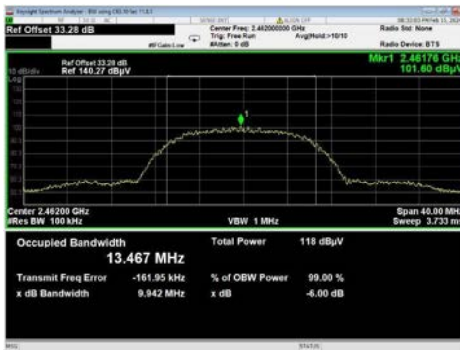
Figure 31 - Bandwidth, WiFi B, High Data Rate, High Channel
