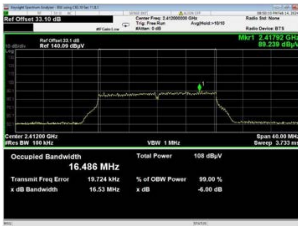
Figure 35 –Bandwidth, WiFi G, High Data Rate, Low Channel
