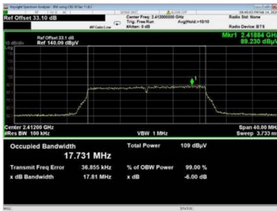
Figure 41 –Bandwidth, WiFi N, High Data Rate, Low Channel
