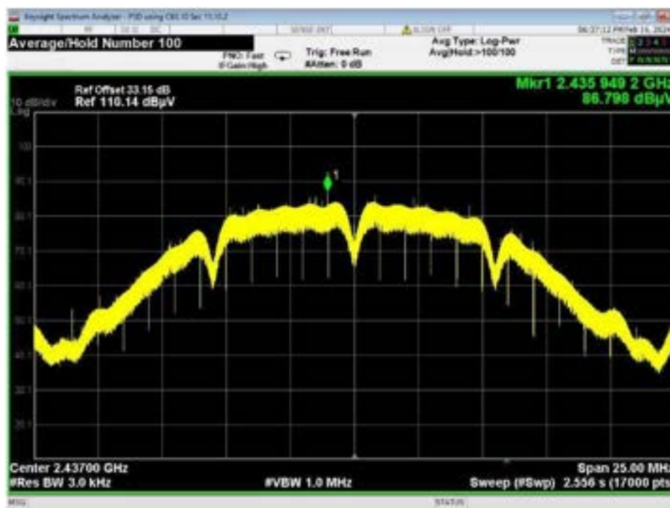
Figure 69 – Radiated EIRP Power Spectral Density, WiFi B, Low Data Rate, Mid Channel
