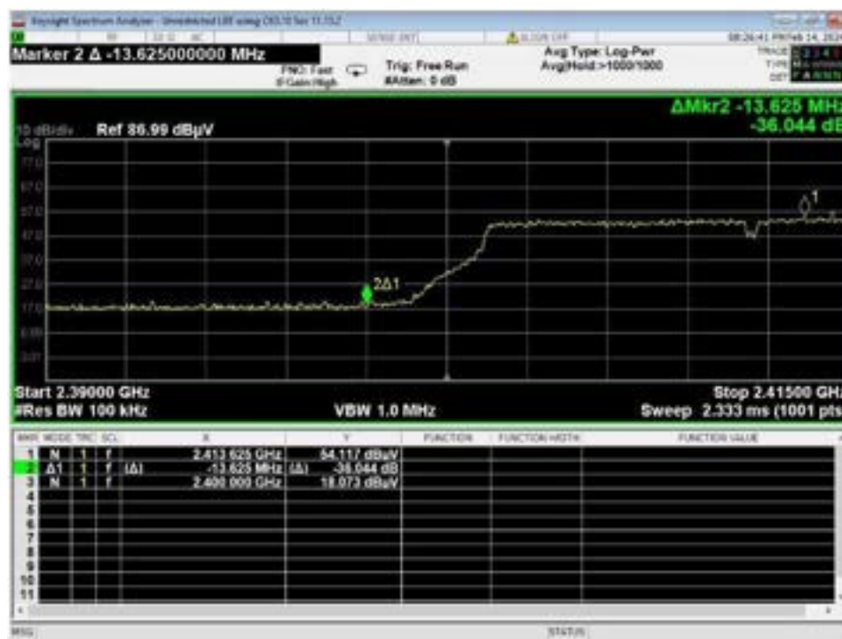
Figure 60 – Band-edge Measurement, WiFi G, Low Data Rate, Low Channel, Unrestricted Frequency
