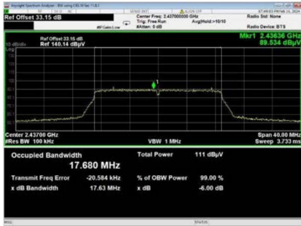
Figure 39 - Bandwidth, WiFi N, Low Data Rate, Mid Channel
