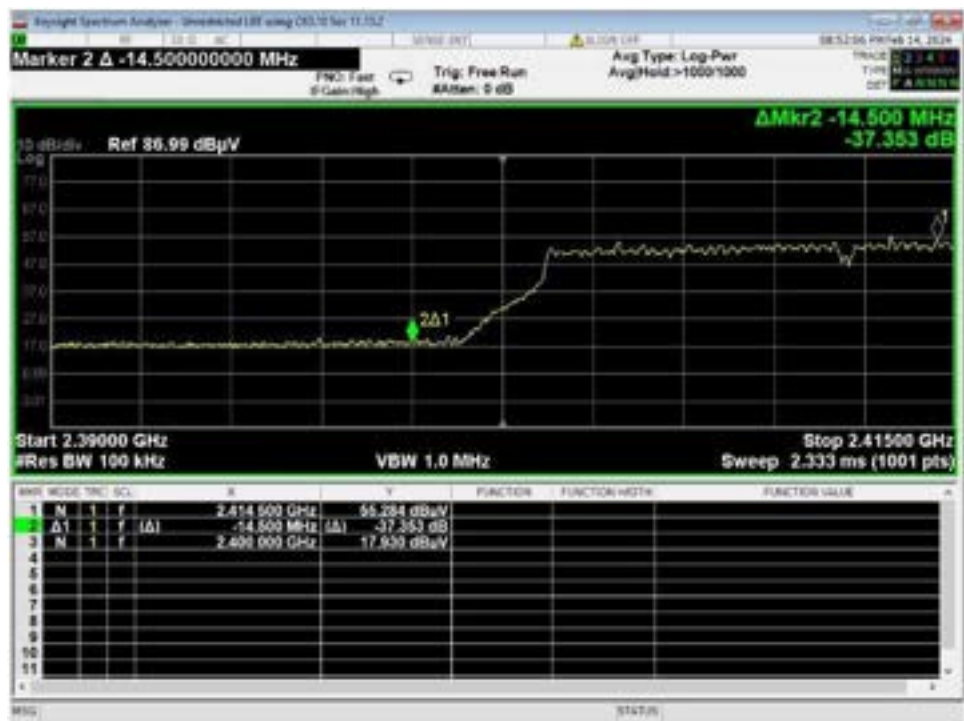
Figure 62 – Band-edge Measurement, WiFi G, High Data Rate, Low Channel, Unrestricted Frequency
