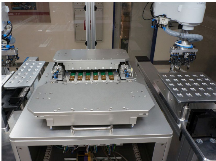
Figure 15: Automatic test equipment for module test
