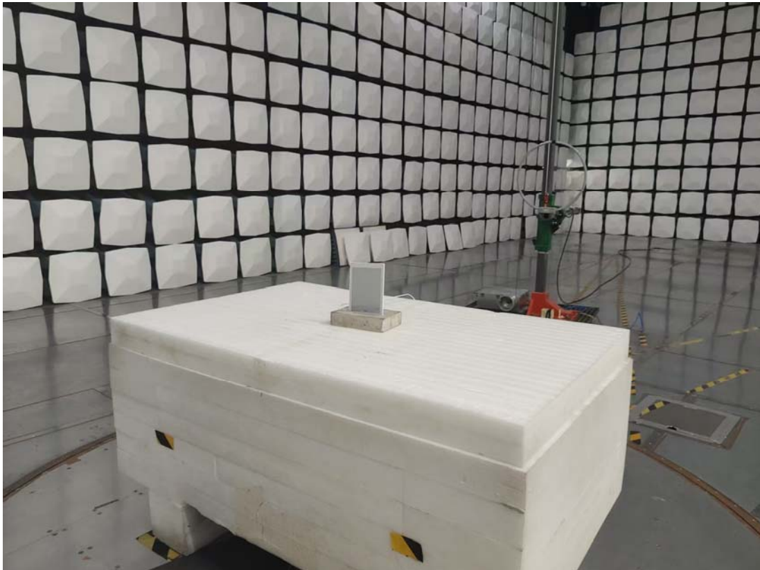
Radiated Emission 9k-30MHz Perpendicular View
