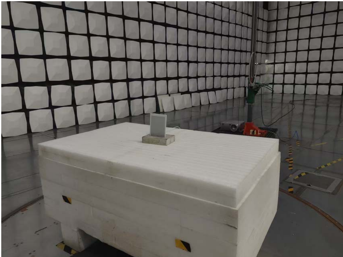
Radiated Emission 9k-30MHz Perpendicular View
