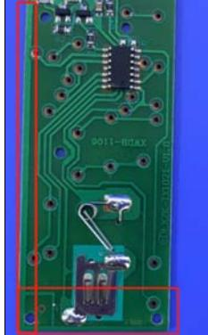
A photograph of a green printed circuit board (PCB) with a red rectangular box drawn around its central rectangular area. The board has various electronic components, including a central integrated circuit, resistors, and capacitors, all mounted on a green substrate. The red box highlights the main body of the PCB, which is the antenna plate mentioned in the report. |
