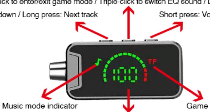
Power on to display battery level, short press volume buttons to display volume, display lights up with any button operation.
