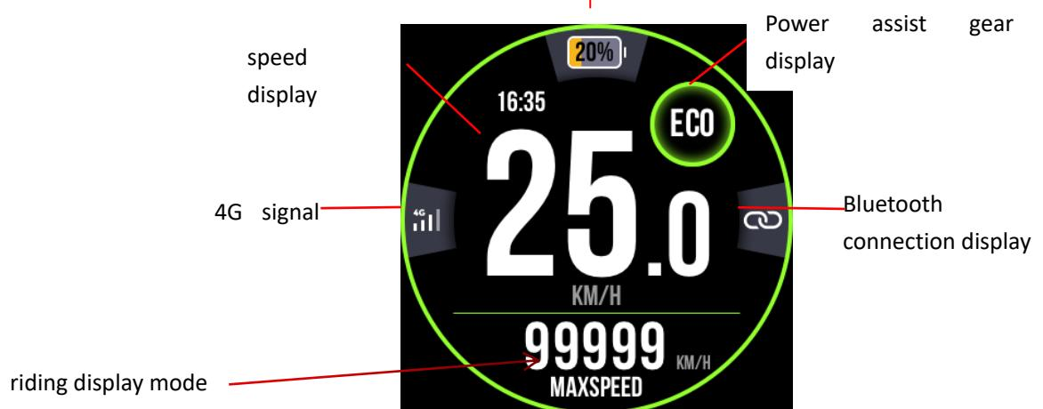
After powering on, the boot logo interface is displayed for 3 seconds. The instrument establishes communication and obtains information normally before entering the normal
