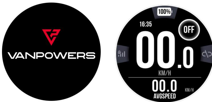
When starting up, the startup logo interface is displayed for 3 seconds. After the communication connection is established, the instrument enters the main interface display state. The instrument uses the information obtained from the controller communication for actual display. (The displayed data information is executed according to the communication protocol provided by the customer)
