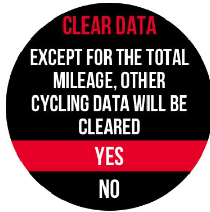
After the data is cleared, the subtotal mileage returns to zero, as does the average speed and maximum speed; the accumulated mileage ODO value is not cleared through any operation on the instrument side and requires professional maintenance tools to clear it.
