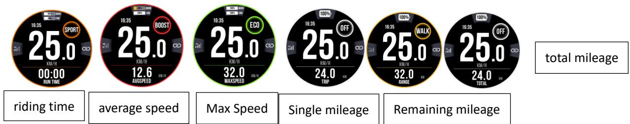
\*If the system does not support the BMS communication function, the instrument cannot obtain accurate RANGE information, and the RANGE item value on the instrument is displayed as ---KM.
