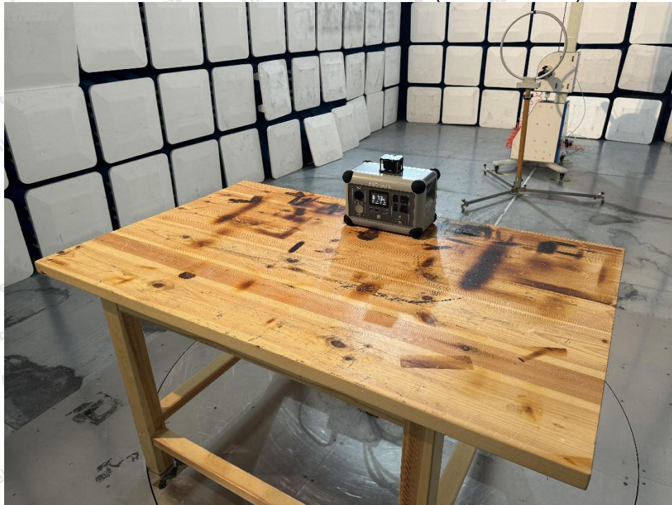
Photo of Radiation Emission Test (below 30MHz)
