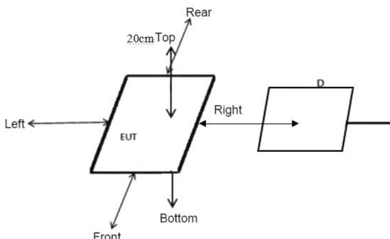
Note: Measurements should be made at 20 cm surrounding the EUT and 20cm above the top surface
