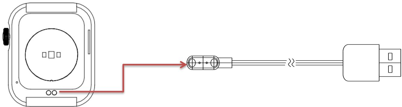
Note: Connect the USB interface to a charger or computer USB interface with an output current of 500mA or above for charging
