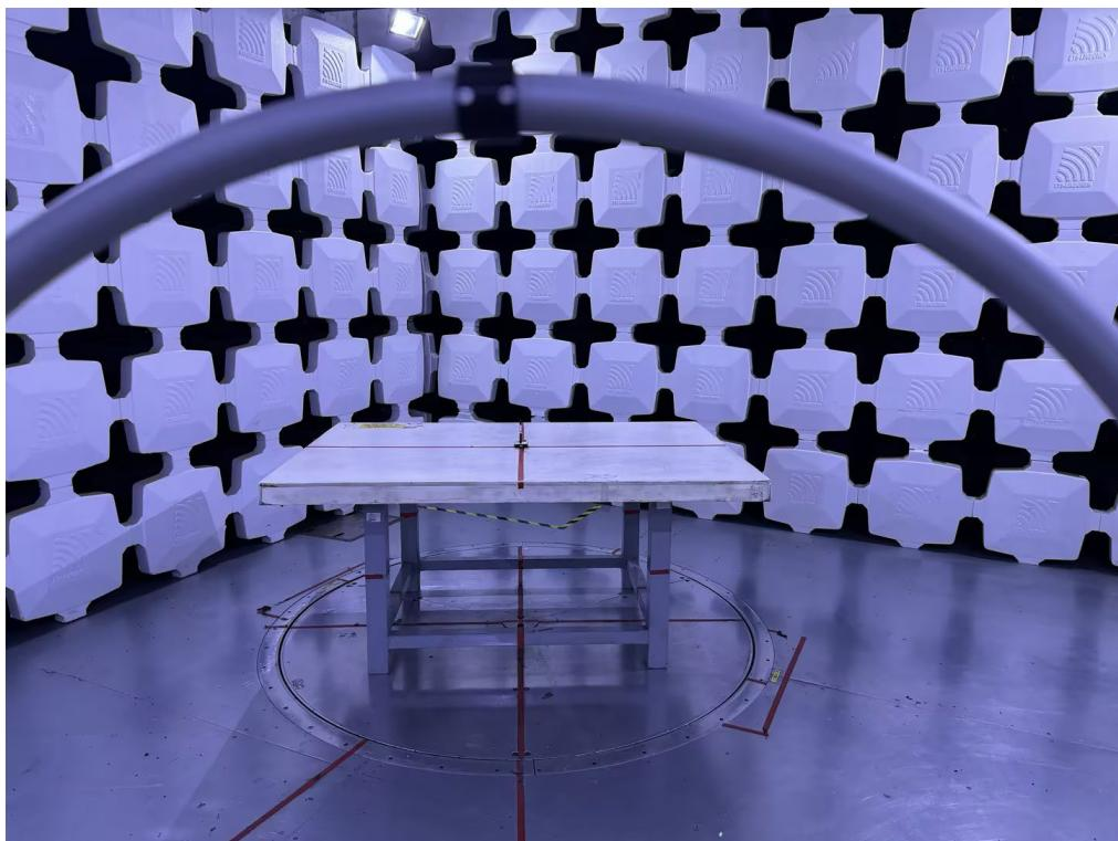
**Radiated Emissions Test Photos****30 MHz to 1 GHz**
