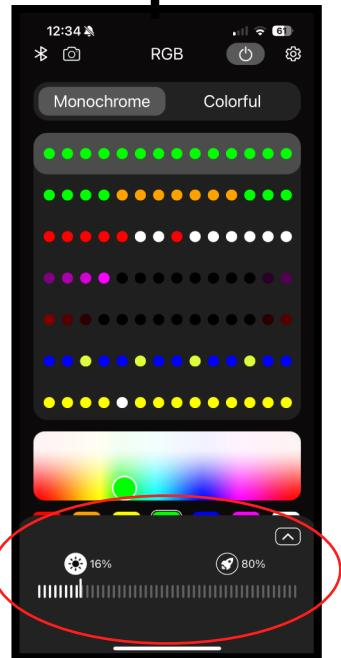
1. BRIGHTNESS CONTROL - When you select this button, it allows you to adjust the brightness of the harness using the slider bar. This feature is very helpful as light can be very bright in enclosed spaces so you will want it to be turned down.
