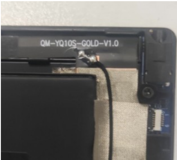
Stick conductive cloth on the copper leakage area of the antenna and ground the screen.
