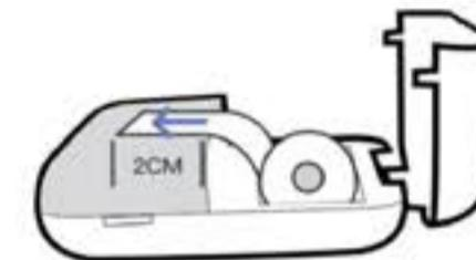
new paper roll in the direction shown. The paper should be put straight and not crooked. (Note: The new thermosensitive paper needs to be exposed to 2 cm of paper bin length so that the machine can absorb paper automatically when the paper bin is shaped)
