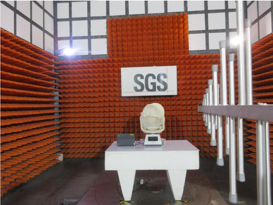
Radiated Spurious Emissions Below 1GHz
