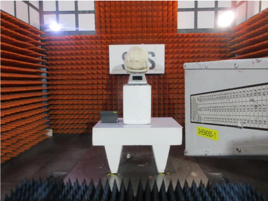
Radiated Spurious Emissions Above 1GHz
