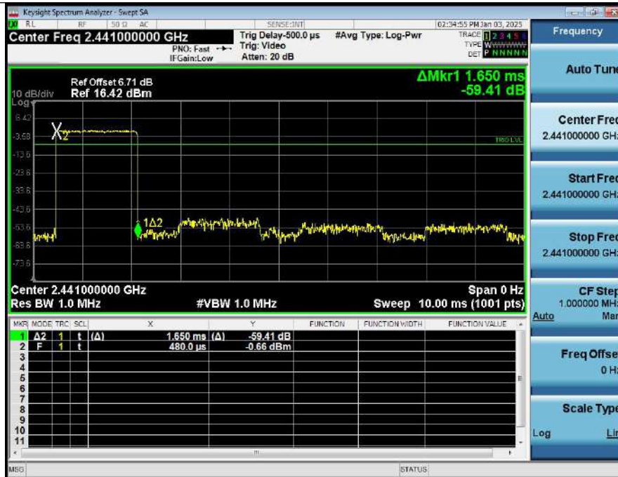
Dwell Time (Hopping) NVNT_ANT1_2-DH3_2441_00_Accumulated
