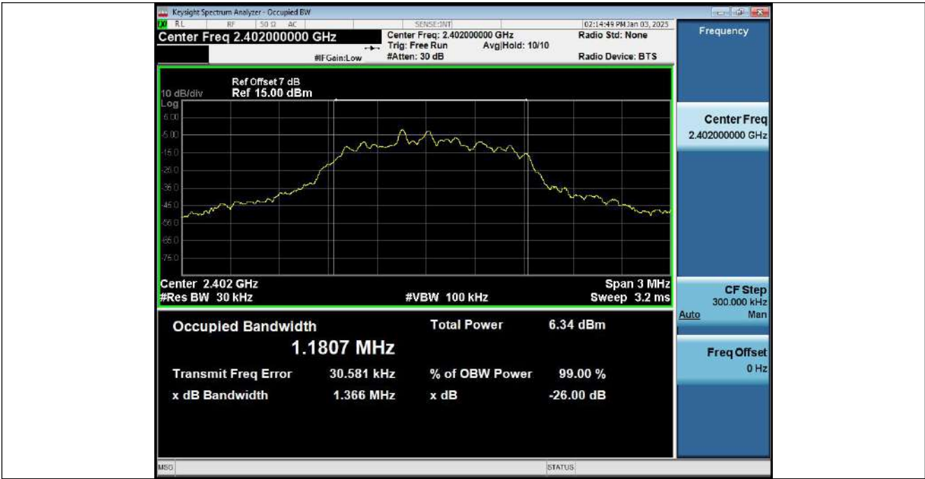
99% Occupied Bandwidth NVNT_ANT1_3-DH1_2441_00
