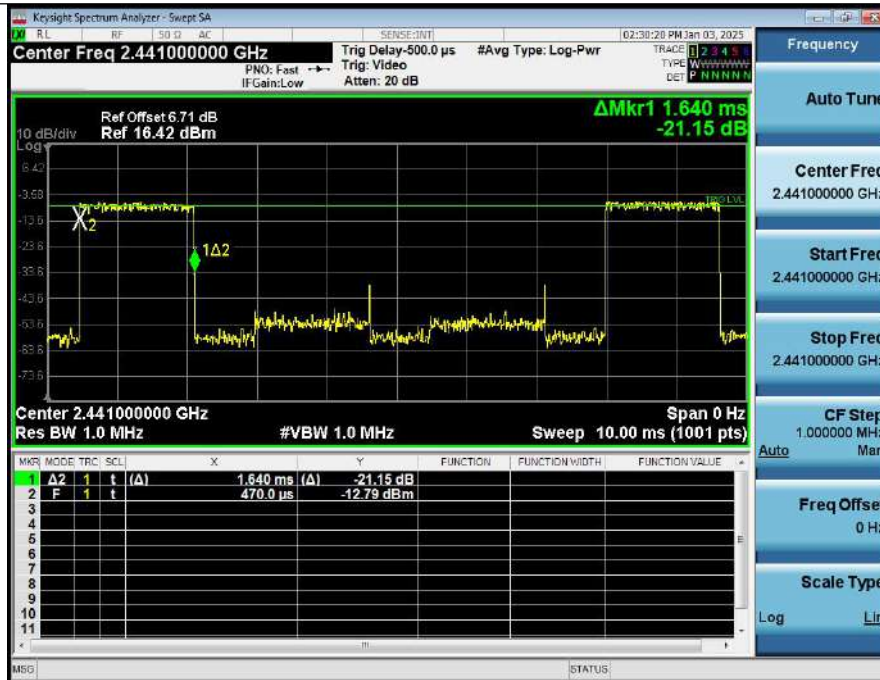
Dwell Time (Hopping) NVNT_ANT1_1-DH3_2441_00_Accumulated
