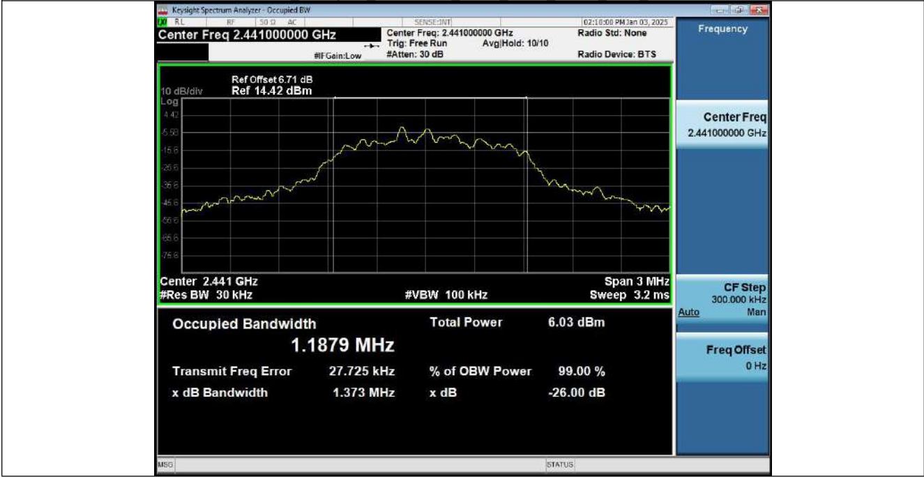
99% Occupied Bandwidth NVNT_ANT1_3-DH1_2441_00
