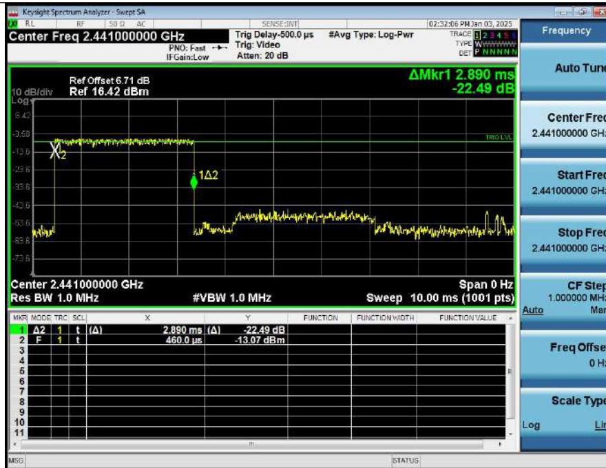
Dwell Time (Hopping) NVNT_ANT1_1-DH5_2441_00_Accumulated
