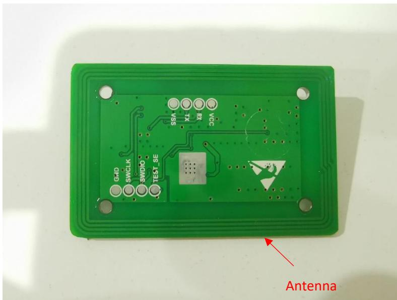
Antenna transmission frequency: 13.56MHz
