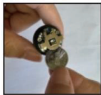
c Insert the new battery and screw the cover on, then install it onto the valve stem (battery text side facing up)
