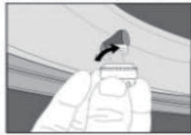
(Fig. b) Quickly tighten the sensor clockwise. Air leakage during installation is normal and will stop once the sensor is fully tightened.
