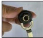
b. Unscrew top cover with wrench
