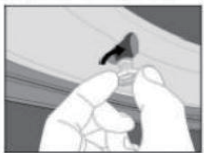
(Fig. a) Clockwise screw the anti-theft nut to the bottom of the tire valve
