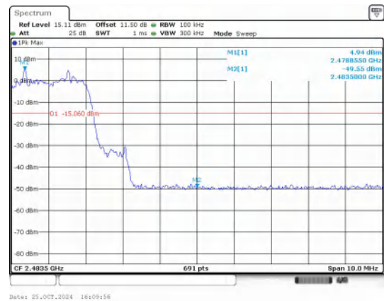
Out Of Band Emission(Right) \pi/4 DQPSK_2-DH5_Channel Hopping
