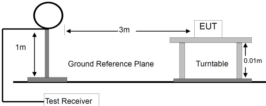
For Radiated Emission 30-1000MHz
