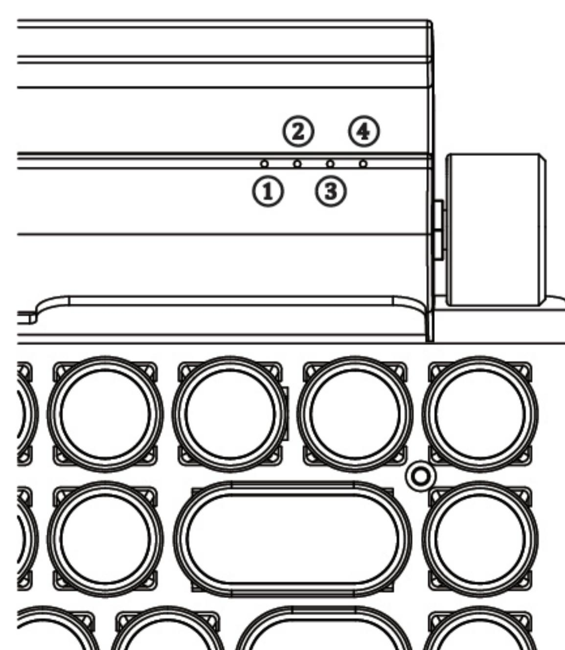
**①Bluetooth/wired mode indicator****Wired mode:** The indicator is red
