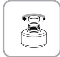
①. Remove the deodorant container and remove the bottle cap by turning it counterclockwise
