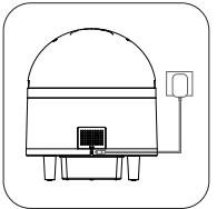
Insert the power adapter port into the rear hole of the product
