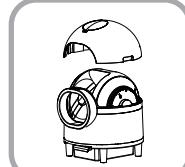
①. Extract the cover from the side of the top cover upward
