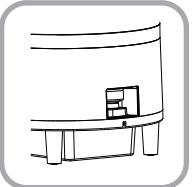
⑥. Install the back cover after the purifier is inserted into place
