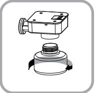
③. The deodorant container is vertically aligned with the mounting port and pressed upward. After opening the sealing port, it is rotated counterclockwise to the purifier
