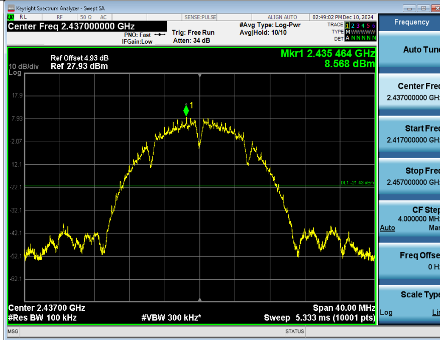
2 Spurious Emission NVNT_ANT1_802_11b_2437
