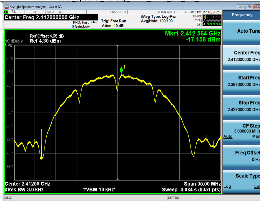
Power Spectral Density_NVNT_ANT2_802_11b_2412
