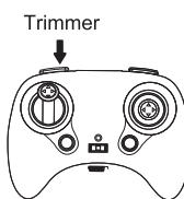
If the helicopter rotates anti-clockwise, long press the trimmer button and push the right joystick to right until the helicopter gets stabilised.
