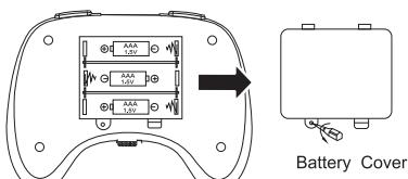
1. Unscrew the battery cover and insert 3 x AAA batteries into the battery compartment according to the correct polarities.
