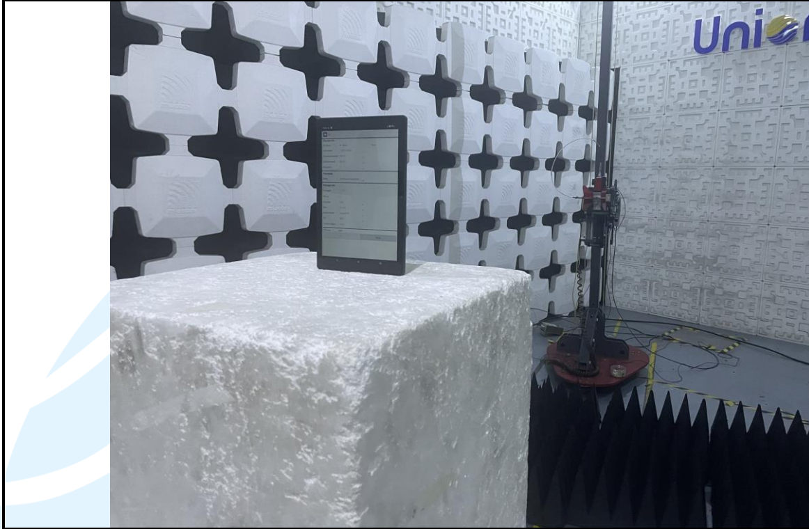
Radiated emission Test Setup (Above 1 GHz)
