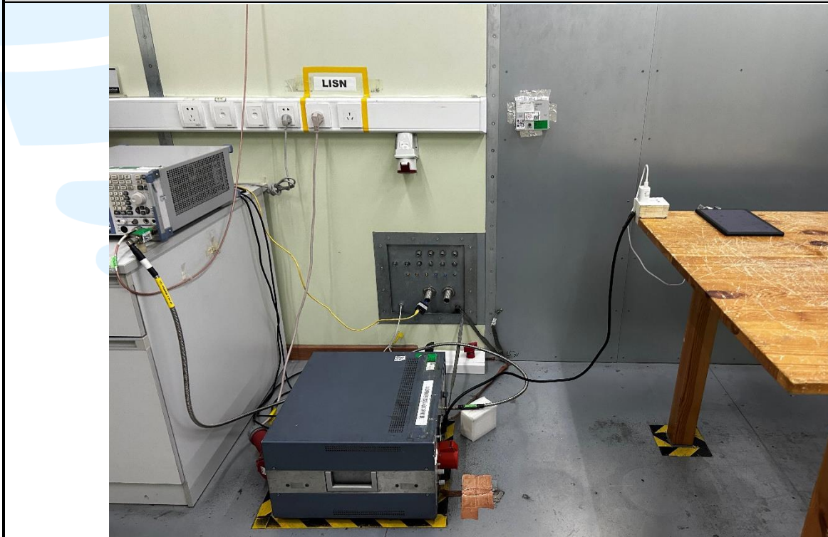
Conducted Emission Test Setup
