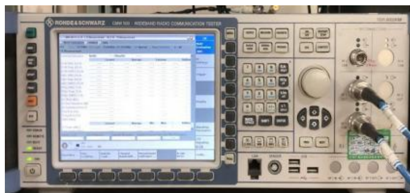
CMW 500 (2G/3G/4G Test Equipment)
