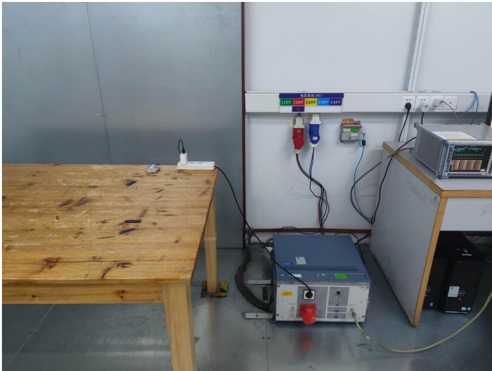
AC POWER LINE CONDUCTED TEST SETUP
